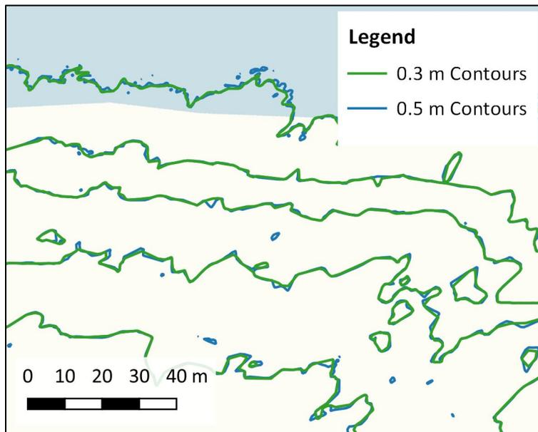
Figure 3: Comparison on 0.3 m contours provided by DOU and 0.5 m contours created from the DEM, plotted at 1.5 m intervals.
