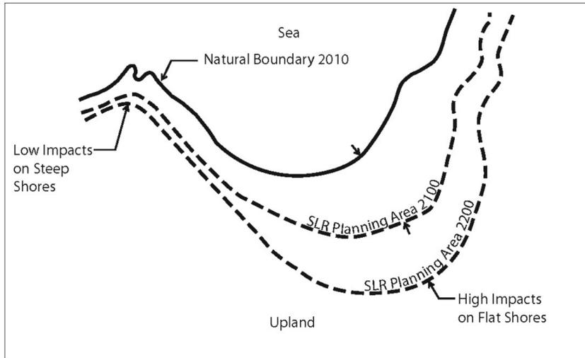
Figure 3: Concept plan of SLR Planning Area varying with terrain (Ausenco-Sandwell, 2011).
