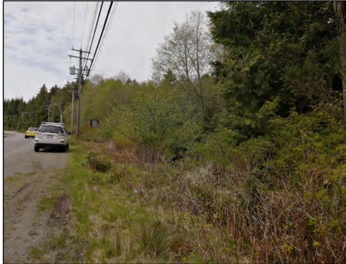
Photo 7: Storm water from road flows overland down this vegetated slope on the north side of Peninsula Road, and storm drains *appear* to discharge into this area.
